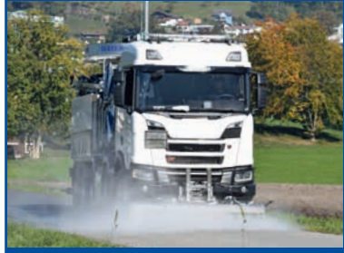
Street cleaning using washing bar with pneumatically actuated swing movement.
