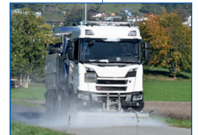
Street cleaning using washing bar with pneumatically actuated swing movement.
